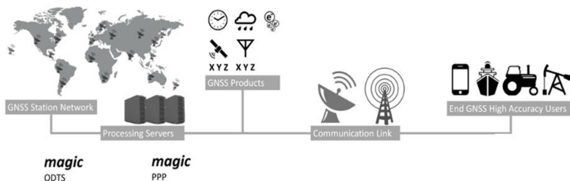
Figure 1: End-to-end PPP chain
