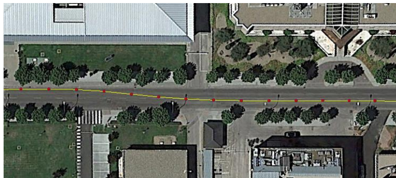
Fig. 12: Lane change detection in urban environment Estimated (red dots) vs. Reference (yellow line) trajectory
