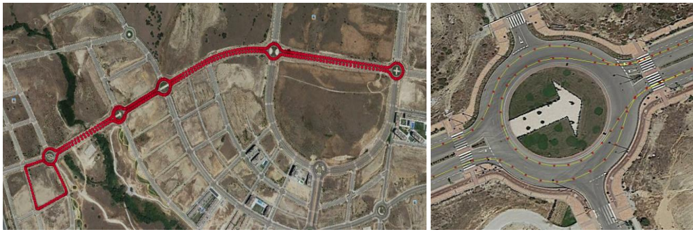
Fig. 7: Kinematic open-sky. Left: Estimated trajectory Right: Estimated (red dots) vs. Reference trajectory (yellow line), roundabout close-up
