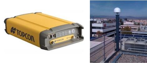
**Figure 8: GAP4 Station: receiver (left) and antenna (right)**
