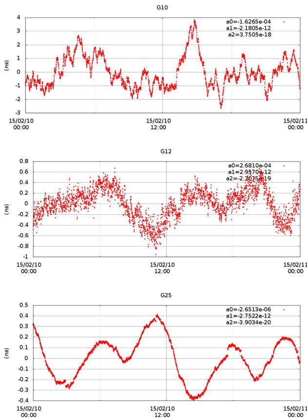
**Figure 5: Detrended GPS clocks for G10 (IIA), G12 (IIR), G25 (IIF)**
