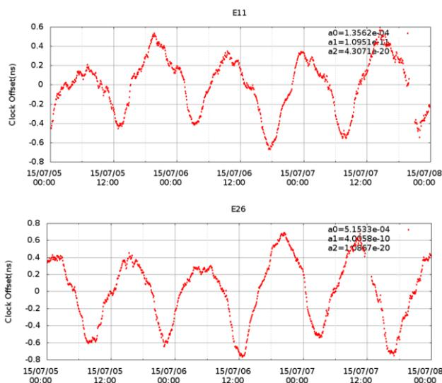
Figure 10 Detrended Galileo clocks for E11 and E26.
