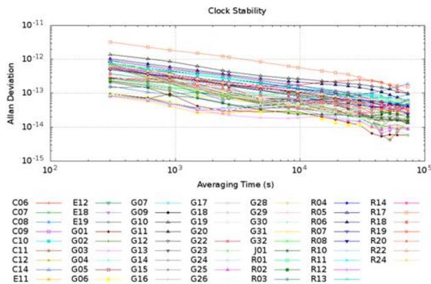
**Figure 1: GNSS ADEV based on *magicGNSS*' estimations**
