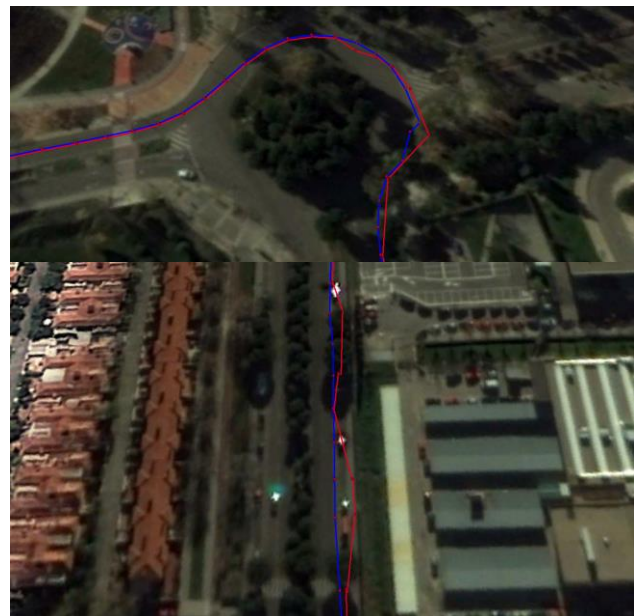
Figure 15 PPP performance improvement due to the addition of Galileo to the GPS+GLONASS solution
