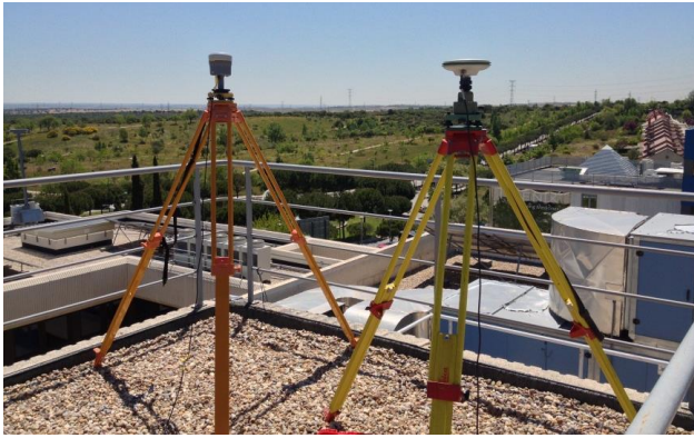
Figure 9 R10 Trimble receiver placed at GMV’s roof
