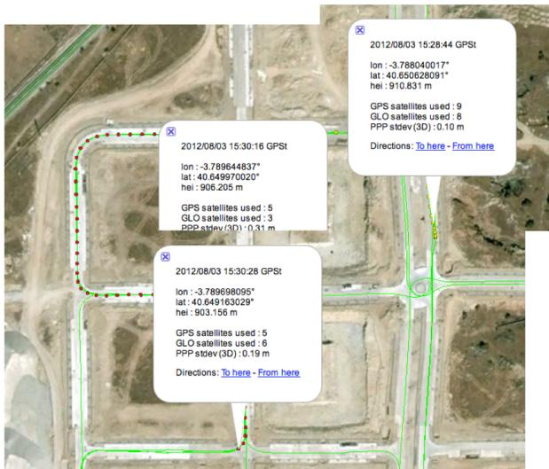
**Figure 18 Impact of satellite loss – test trajectory**
