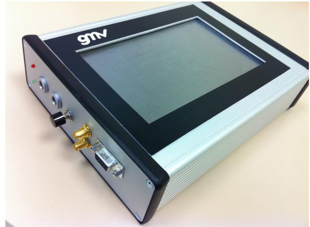
**Figure 7 The PPP user terminal prototype**
