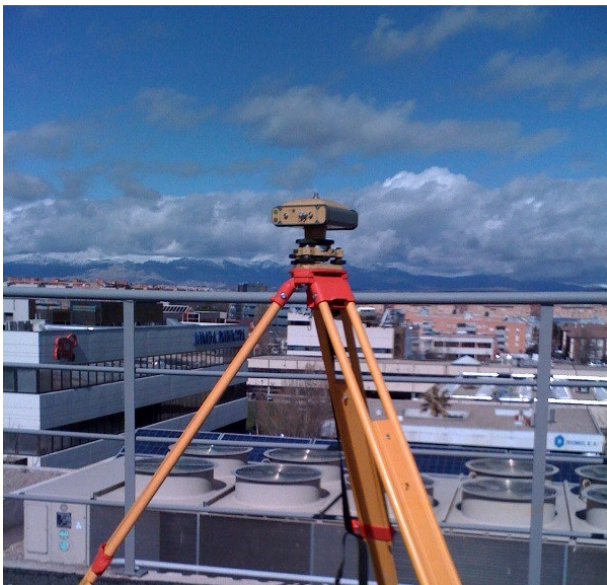
Figure 11: Topcon Hyper receiver
