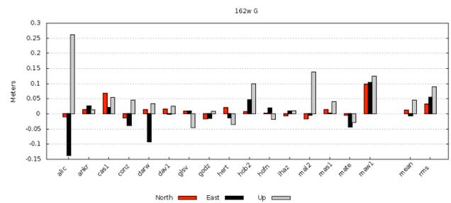
**Figure 18: GPS-only position error in 1 hour**
