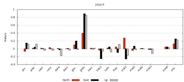
**Figure 19: GLONASS-only position error in 1 hour**
