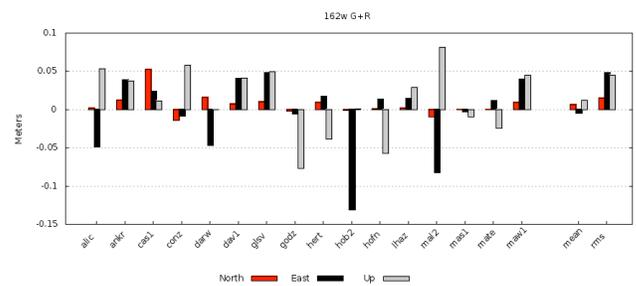
**Figure 20: GPS+GLONASS position error in 1 hour**
