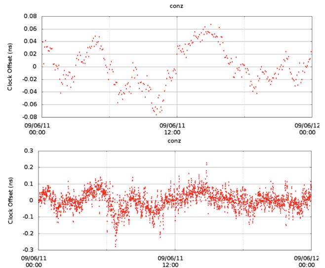
**Figure 21: CONZ station clock using a 5-min data rate (above) and a 30-sec data rate (below)**
