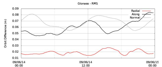
**Figure 9: Orbit comparison with IGS (vs time)**
