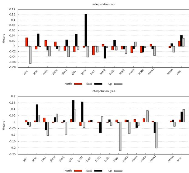
**Figure 22: Effect of clock interpolation in 1-hour positioning (above: 5 min; below: 30 sec)**
